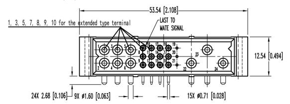
Connector pin Layout (on the backplane)(view from rectifier plugging side):
